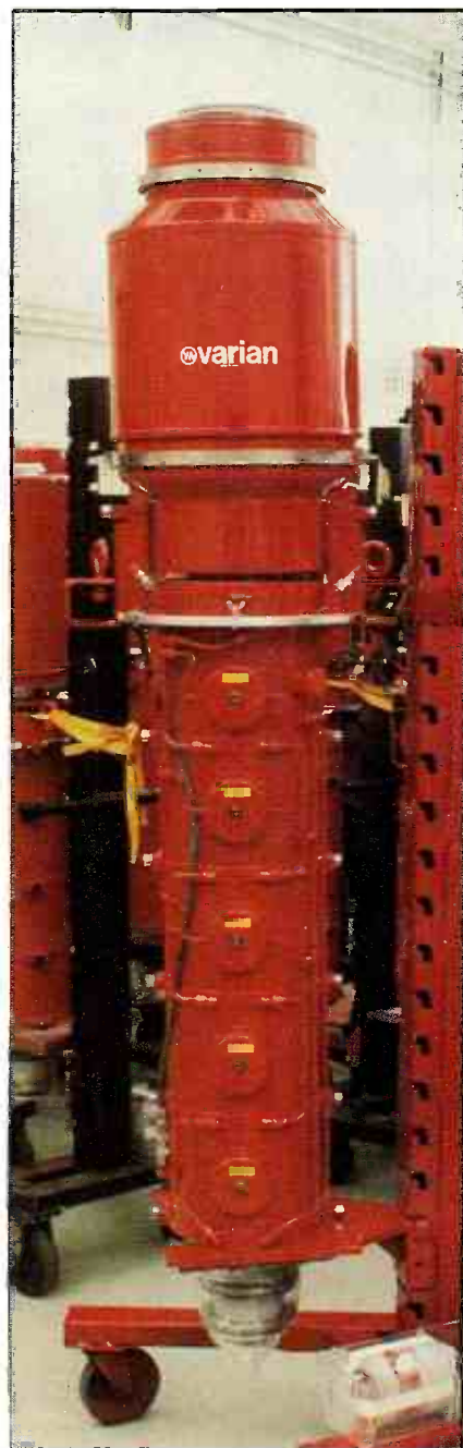
An integral cavity klystron showing RF region structure and cooling tubing.
